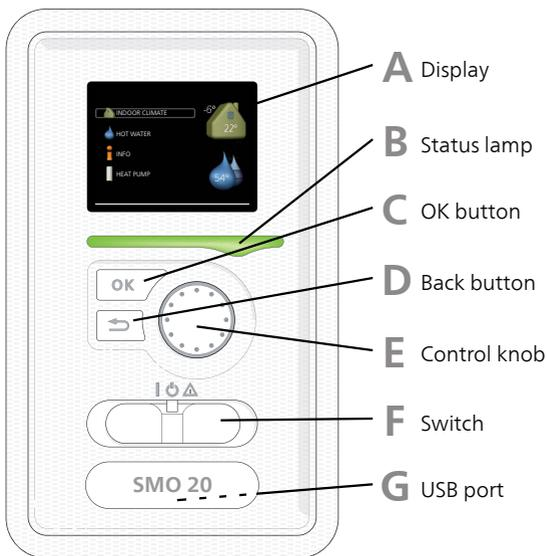
There is a display unit on the front of the control module, which is used to communicate with SMO 20. Here you:
