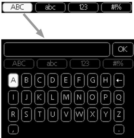
Depending on the menu, you can gain access to different character sets which you can select using the control knob. To change character table, press the Back button. If a menu only has one character set the keyboard is displayed directly.
