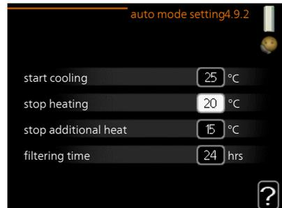
When the operating mode is set to "auto", the control module selects when start and stop of additional heat and heat production is permitted, depending on the average outdoor temperature. If the heat pump has the integrated cooling function and it is activated in the menu you can also select the start temperature for cooling.
