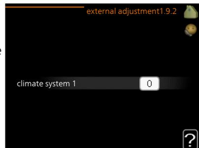
Connecting an external contact, for example, a room thermostat or a timer allows you to temporarily or periodically raise or lower the room temperature while heating. When the contact is on, the heating curve offset is changed by the number of steps selected in the menu. If a room sensor is installed and activated the desired room temperature (°C) is set.
