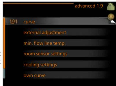
the heating curve and read off how the supply temperature changes at different outdoor temperatures here. If there is access to cooling the same settings can be made for the cooling curve.
