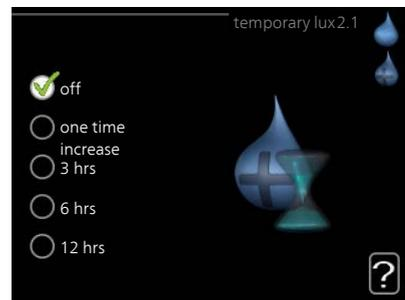
When hot water requirement has temporarily increased this menu can be used to select an increase in the hot water temperature to lux mode for a selectable time.
