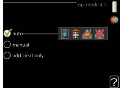
The control module operating mode is usually set to "auto". It is also possible to set the control module to "add. heat only", when only additional heat is used, or "manual" and then select what functions are to be permitted.
