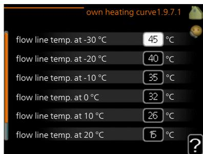
Create your own heating or cooling curve here, by setting the desired supply temperatures for different outdoor temperatures.
