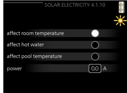
Here you set whether you want EME 20 or EME 10 to affect the room temperature and / or the hot water and / or the pool temperature. How much this is affected depends on how much electricity the solar panels produce. The heat pump therefore has 4 operating mode for this.
